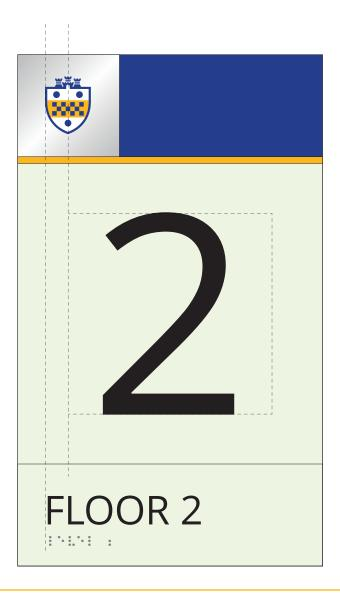
The Stair ID is an IFC (International Fire Code) and IBC (International Building Code) required identification sign. They identify the stairwell and its exit.
